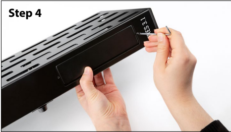
Insert the supplied screws and hand-tighten them to secure the Slot Cover.
